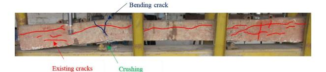
Fig. 13 – Typical view of sleeper after failure (Severe damaged)
