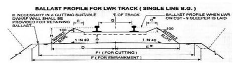
Fig. 2 – Ballast profile track slab
