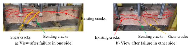
Fig. 18 – Typical view of sleeper after shear failure
