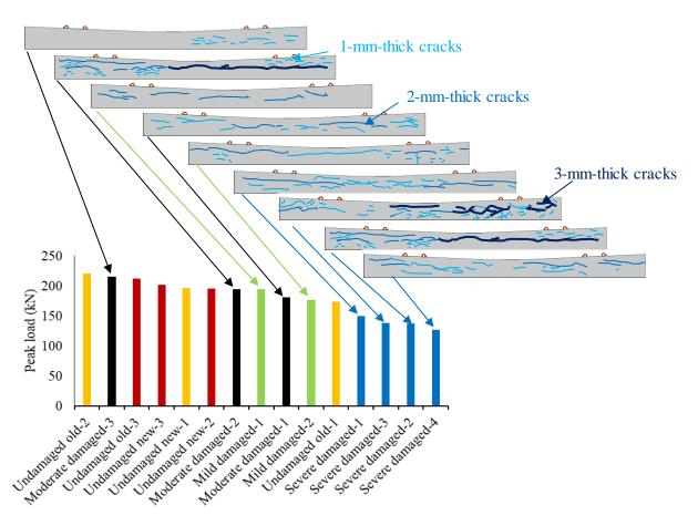
Fig. 14 - Side view - comparison of capacity in damaged sleeper
