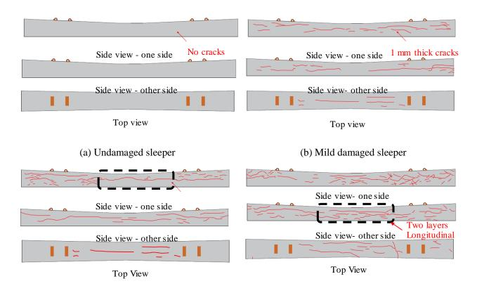
(c) Moderate damage sleeper (d) Severe damage sleeper Fig. 11 – View of crack patterns of sleepers before loading
