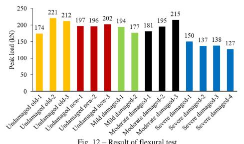
Fig. 12 – Result of flexural test
